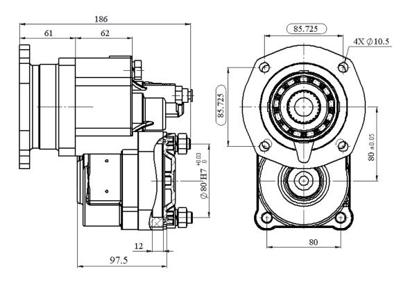
PTO WITH PUMP, PTO WITH FLANGE COMBINATION WILL BE SUPPLIED AS PER CUSTOMER REQUIREMENT
