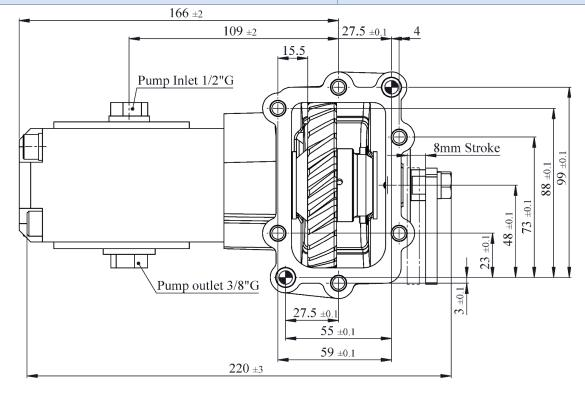
PTO WITH PUMP, PTO WITH FLANGE COMBINATION WILL BE SUPPLIED AS PER CUSTOMER REQUIREMENT
