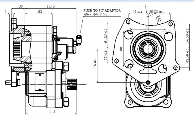
PTO WITH PUMP, PTO WITH FLANGE COMBINATION WILL BE SUPPLIED AS PER CUSTOMER REQUIREMENT
