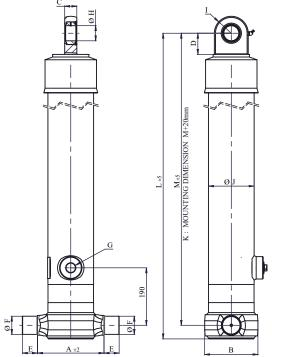
201 mm В mm 176 40 mm D **70** mm mm 50 mm 60 **BSP** 1" mm 50 mm 56 152 mm 1530 mm 1556 mm  $\mathbf{M}$ : 1511 mm
