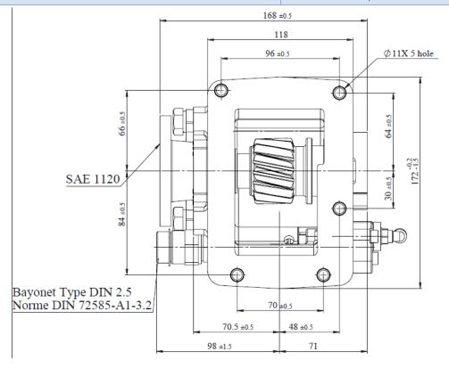
PTO WITH PUMP, PTO WITH FLANGE COMBINATION WILL BE SUPPLIED AS PER CUSTOMER REQUIREMENT
