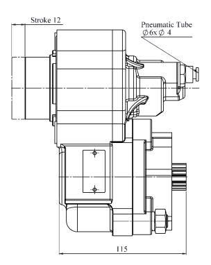
PTO WITH PUMP, PTO WITH FLANGE COMBINATION WILL BE SUPPLIED AS PER CUSTOMER REQUIREMENT **INTERPUMP** HYDRAULICS
